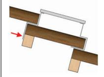
Space & attach brackets to Solar Panel so they align with the valley of the tiles.
