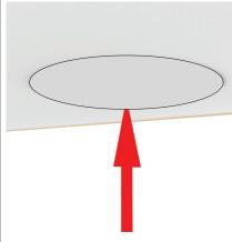
Be aware of any obstructions or trusses where you want to located LED panel. Mark & cut plaster using template provided using a plaster knife
