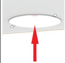
Connect cable from the solar collector. Fold one side spring clips located on the LED panel first and then do the same for the other side
