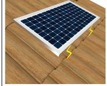
Attach top-brackets to the roof battens. Fold bottom-bracket around and under the tile at the bottom. Run cable into roof cavity
